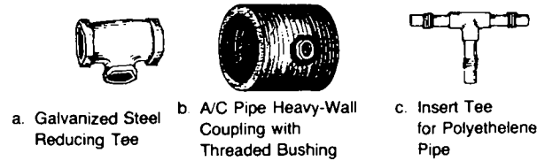
Figure 1. Service Tees Installed During Construction
