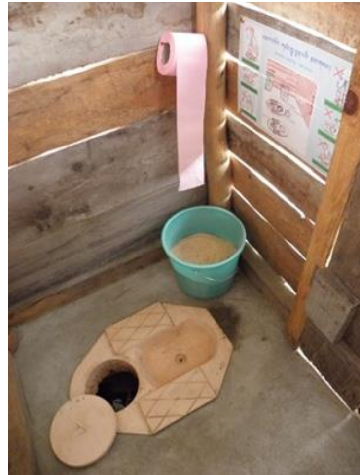
Exterior and interior view of Double-Vault UDDT by Ministry of Health, Bhutan
