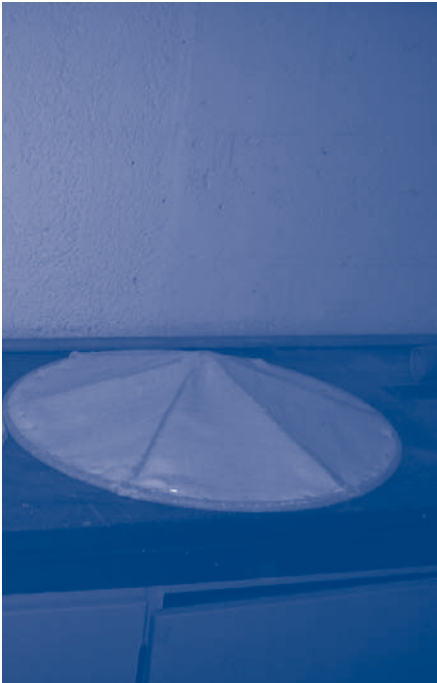
Figure 9.2. Self cleaning cloth filter (Picture: D.B. Martinson)
