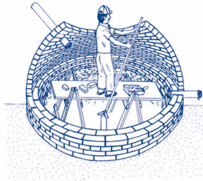
Making the brick dome
