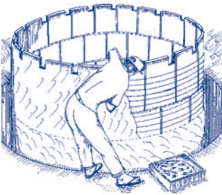
Plastering the outside
