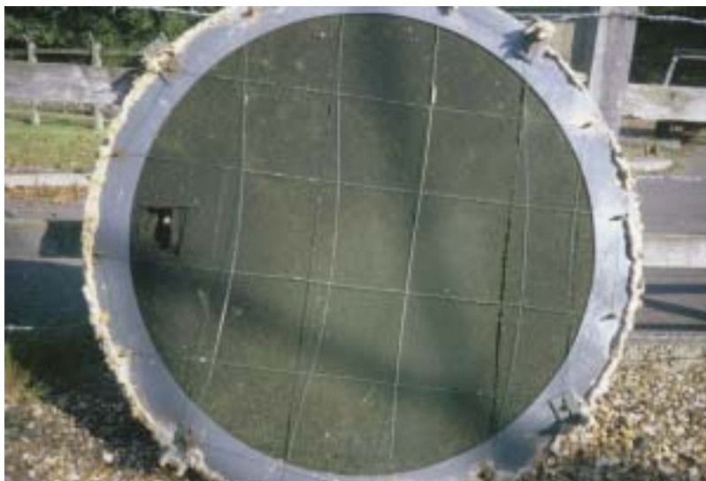
Plate 4.16: Surface mat installed onto a pilot scale SSF bed at Shalford (Surrey, UK)
