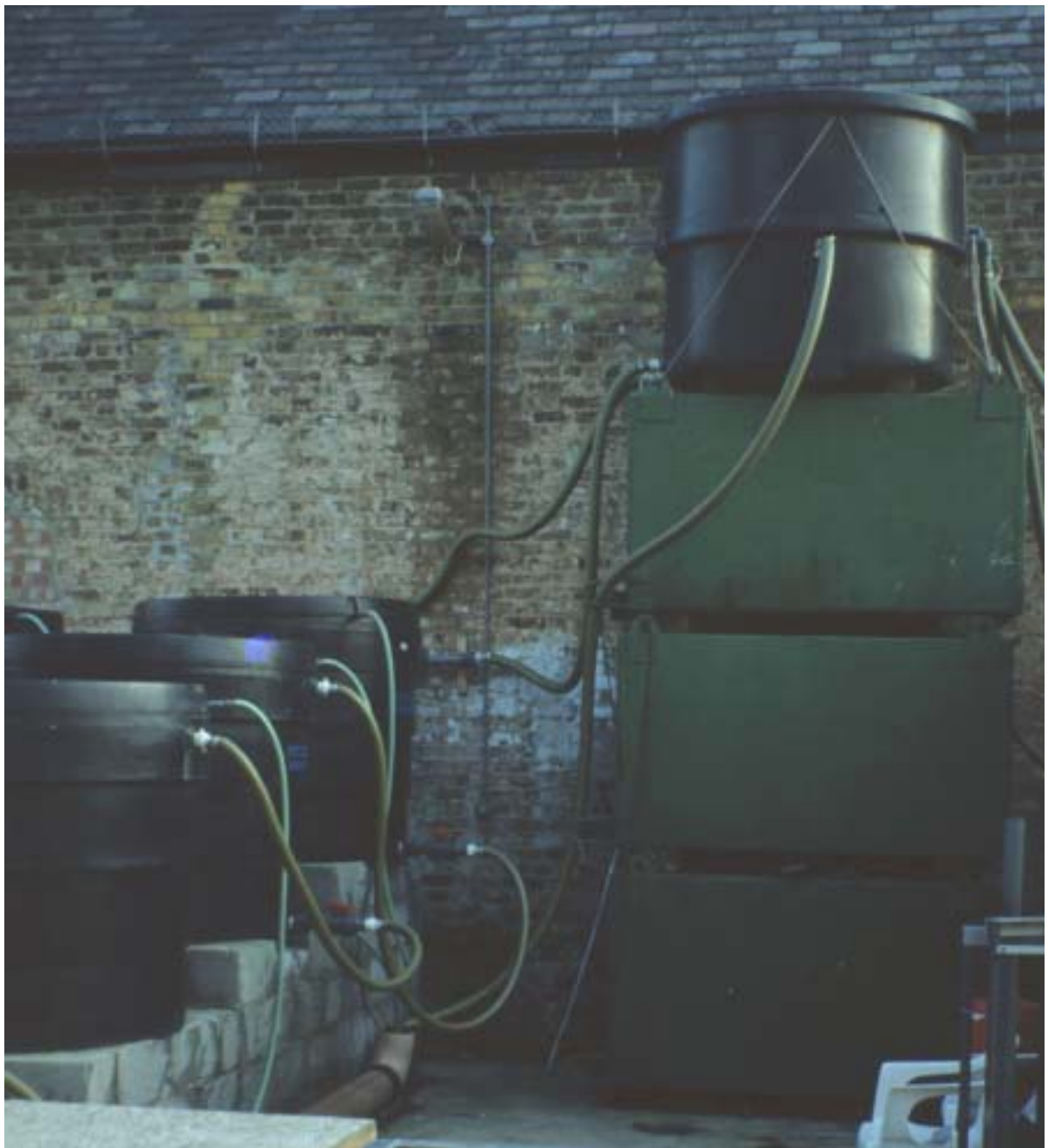
Plate 4.1: Header tank and filter tanks in series (an MSF system), operating under gravity flow at a pilot plant at Surbiton (London, UK).
