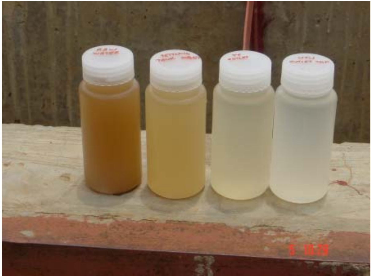
Plate 5.9: Water quality improvement throughout the multi-stage treatment system at the Nyabwishongwezi Water Treatment Plant (Umatara, Rwanda) on 05/Oct/2002. From left to right: raw water tank inlet: 647NTU, raw water tank effluent: 220NTU, pre-filter effluent: 40.2NTU, and slow sand filter effluent: 12.2 NTU (Dorea et al , in press 2004).
