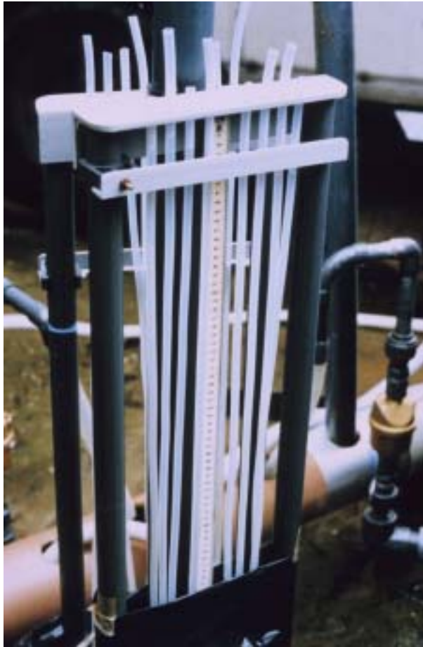
Plate 4.12: Manometer tubes and the scale used to measure headloss between tapings, for a pilot scale filter at Surbiton (London, UK)
