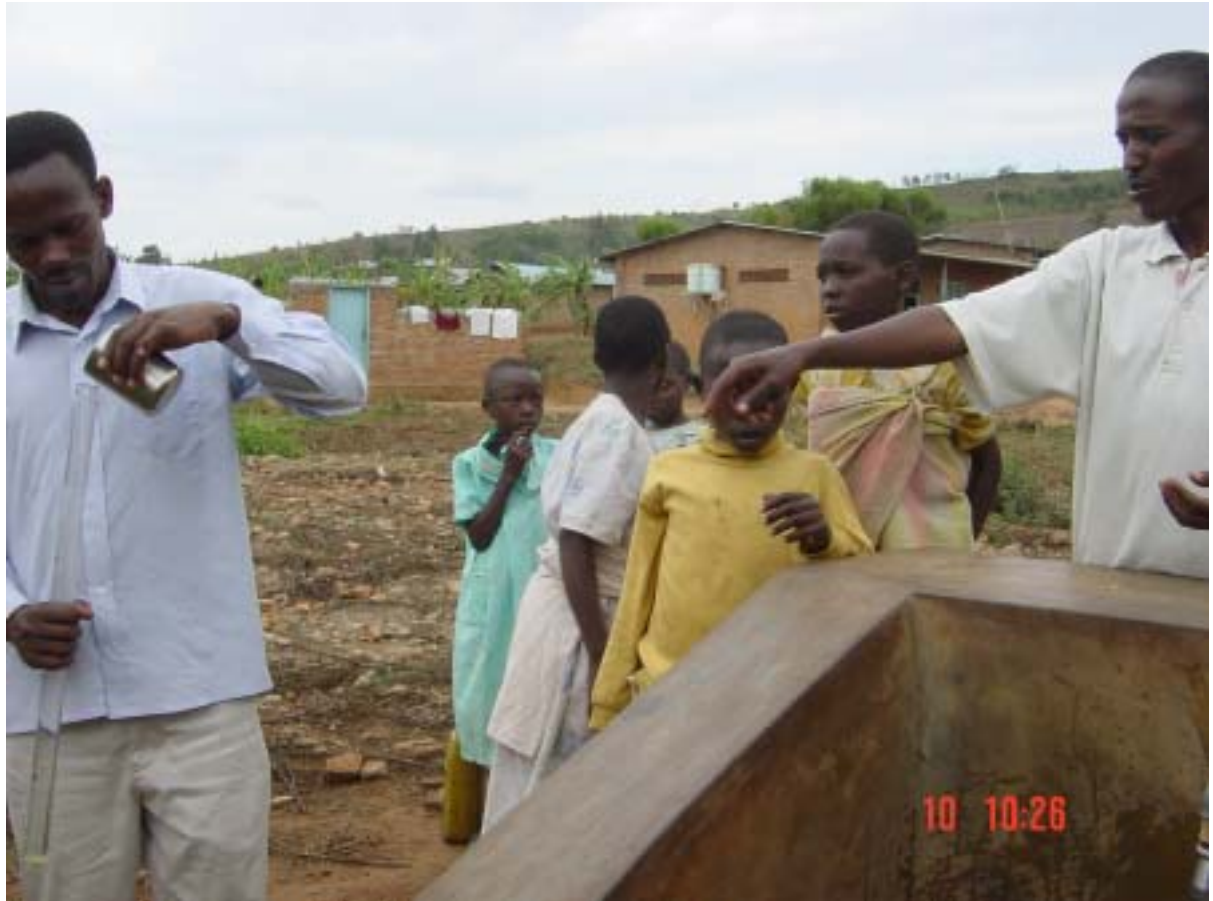
Plate 5.8: Measuring treated water turbidity, using a turbidity tube, at the tap stand at the Nyabwishongwezi Health Centre, Umatara, Rwanda.
