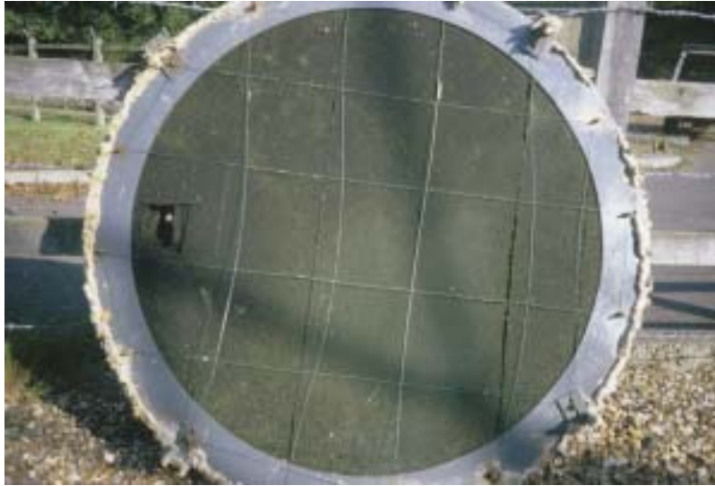
Plate 4.6: Surface Mat Ready for Installation onto a pilot scale SSF at Shalford, Surrey, UK (Plate 4.5)
