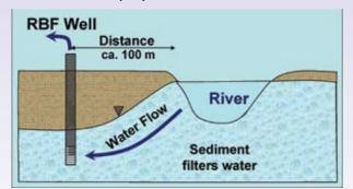
Riverbank filtration operates by extracting water from the wells located near the rivers. Most of the extracted RBF water originates from the river. Contaminants, like bacteria and toxic metals, are removed by overlapping natural processes. Hence, RBF does not require chemicals or heavy maintenance.
