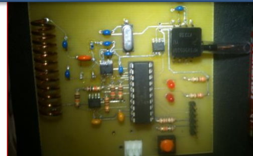
Tank sensor and testing systems
