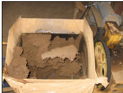
Photo 5-3 Mixing in a Mortar Mixer, Nicaragua (Rayner 2006)
