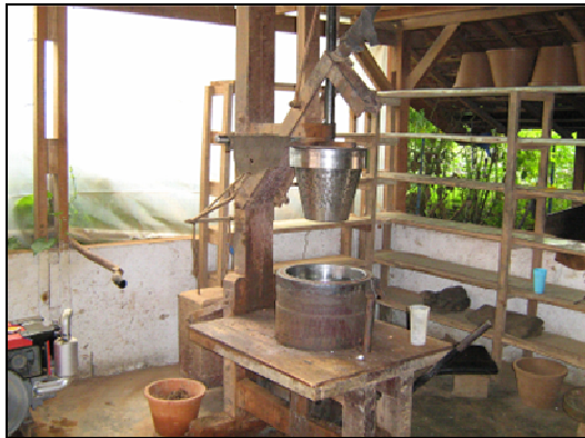
Photo 5-5 Filter Press with aluminium mould, Indo-2 (Pelita 2009)
