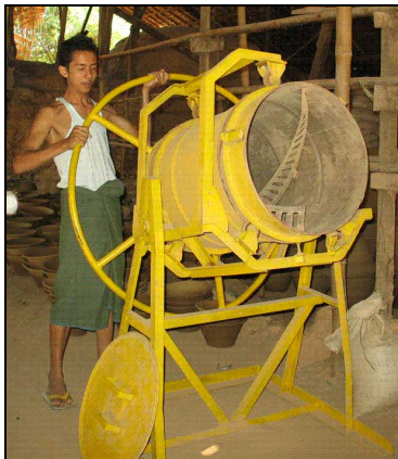
Photo 5-2 Mixing Dry Materials in a Drum Mixer, Myanmar (Thirst-Aid 2009b)
