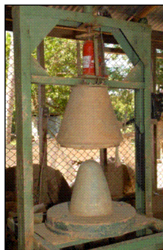
Photo 5-8 Filter Press with cement mould, DR (FilterPure 2009)
