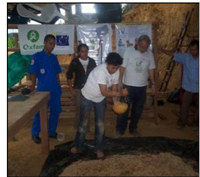
Photo 5-4 Manual Mixing, adding water to filter mixture, Colombia (Asopafin 2009)
