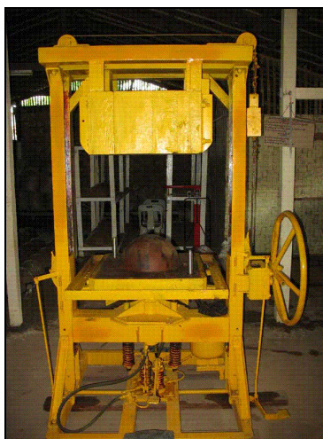
Photo 5-7 Filter Press with wood mould, Myanmar (Thirst-Aid 2009b)
