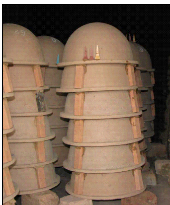
Photo 5-10 Filters Stacked for Firing, Myanmar (Thirst-Aid 2009b)
