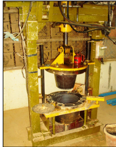
Photo 5-6 Filter Press with cast-iron mould, Cam-1 (IDECambodia 2009)
