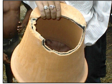
Photo 2-66 Example of Carbon Line in Filter Walls (Source: Unknown)
