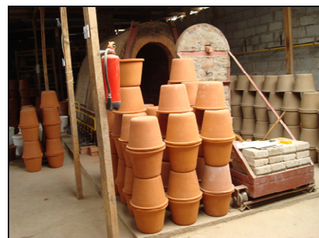
Photo 5-12 Kiln and Fired Filters, Yemen (SilverFilterCompany 2009)
