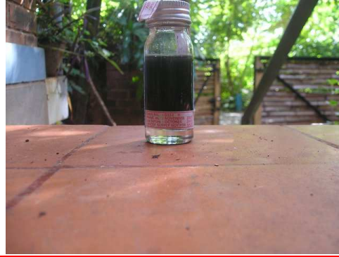
Fig 16 & 17: H2S Strip test bottle. Fill it with water. If the water turns black it needs to be treated
