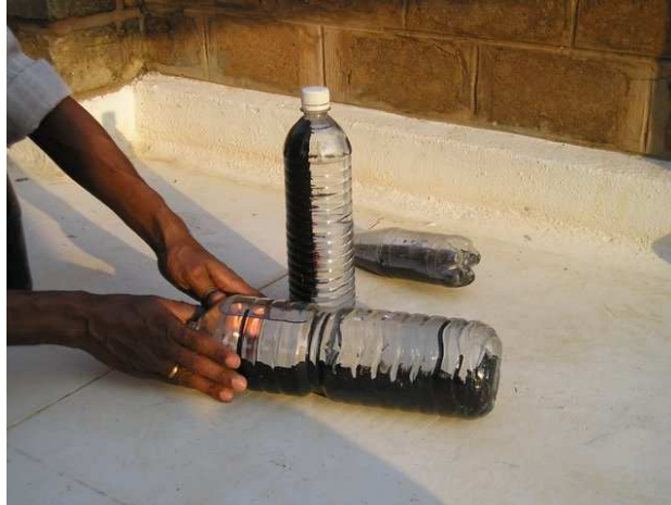
Fig 19: Solar disinfection or SODIS using a bottle painted half black
