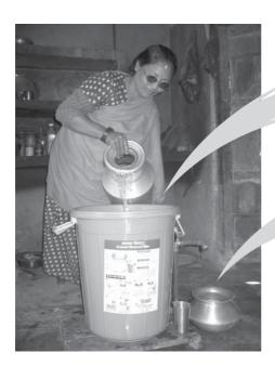
Pour water into top basin. Water will pass through filter and flow up the pipe
