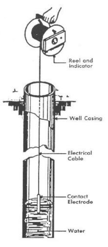
After the operator has measured the static level of the water in the well, the pump should be run for a time to let the water stabilize and then the pumping level should be taken. It is also important to measure the flow in gallons per minute (gpm) that the pump is producing.
