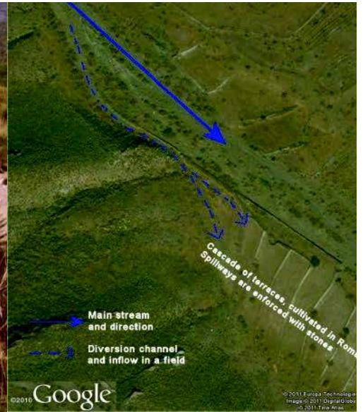
Above left: Water flowing through a traditional channel system ( acequia ) towards almond terraces. (Photo: Joris de Vente) Above right: Aerial view of a traditional water harvesting system ( boquera ) in SE-Spain. (Photo: Google)
