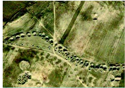
Aerial view of a qanat system in Iran with the access shafts forming a trail towards a village. (www.livius.org)
