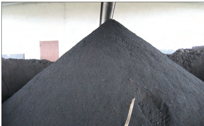
Dewatered Class-A biosolids (31% DS). Photo by Cambi AS
