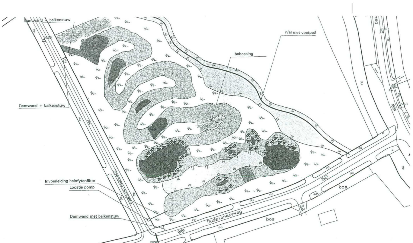
Figure 5.57 A 'natural' constructed wetland Sint Maartensdijk
