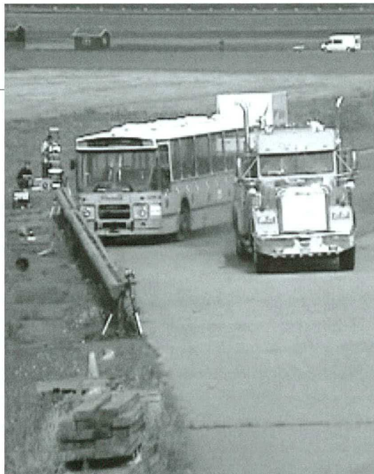
Figure 8.32 Collision test on timber crash barrier
