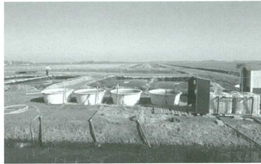
Figure 5.56 Test facilities on Texel. On the foreground the four 2 m 3 mesocosms, behind the four 25 m 3 ponds. At the background the Eversteekoog constructed wetland.
