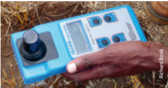
Picture 9: Hand-held turbidity meter
