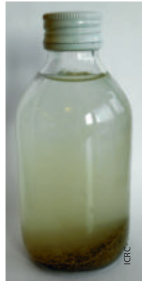
Picture 10: Evidence of sand production
