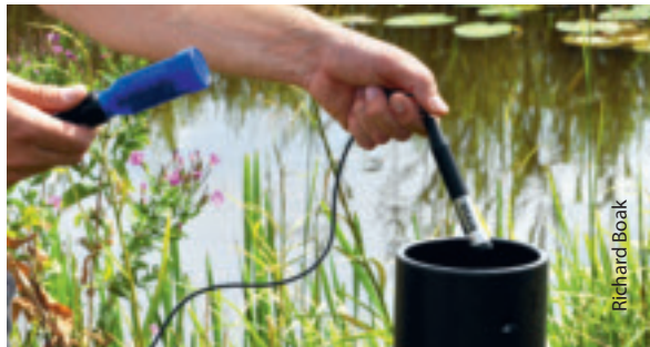
Picture 3: Pressure-transducer installation
