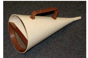
Figure 11: The Marsh funnel viscometer. Top, view showing built-in funnel screen. Bottom, 1000 ml plastic measuring jug with one-quart (946ml) mark
