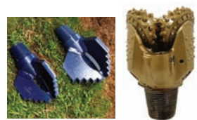
Figure 8: Two common types of drill bits: left, two drag bits; right, a roller cone bit
