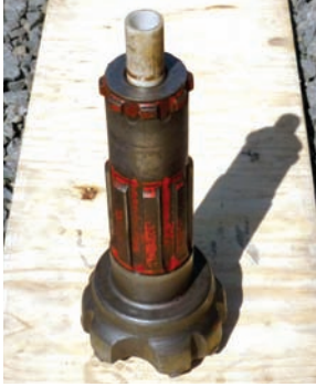
Figure 9: DTH hammer button bits. The hammer body, into which it slides, is not shown
