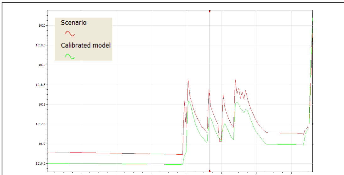
Figure 9.15 Groundwater level calculated by the calibrated model and the scenario with an increase in dam height of 0.75 meter as calculated in the riverbed upstream of the Kwa Ndunda sand dam
