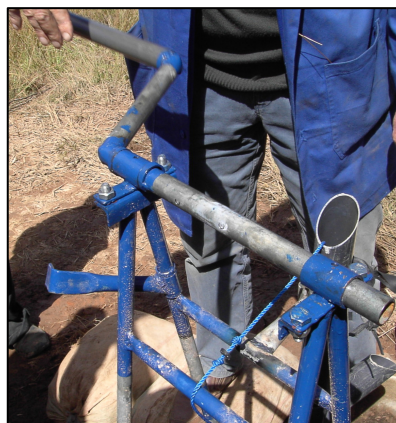
Bushings exactly in line
