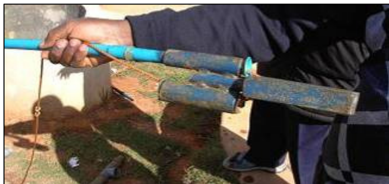
A painted guide box (even than rust may occur. Check regularly)
