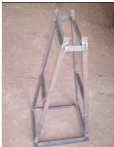
A-model structure jig
