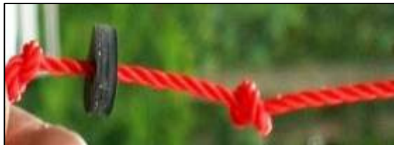
A rubber piston on a rope, between two knots
