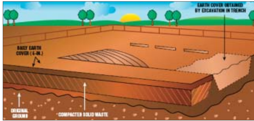
Trench Method of building a sanitary landfill
