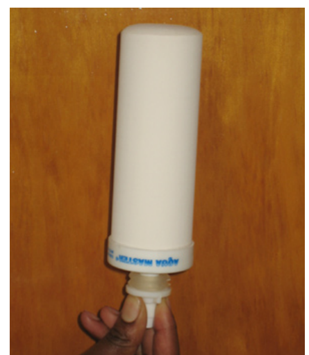
Photos 7: A combined defluoridation filter (above and middle) and the ceramic candle (below). (Source: CDN et al., 2007)
