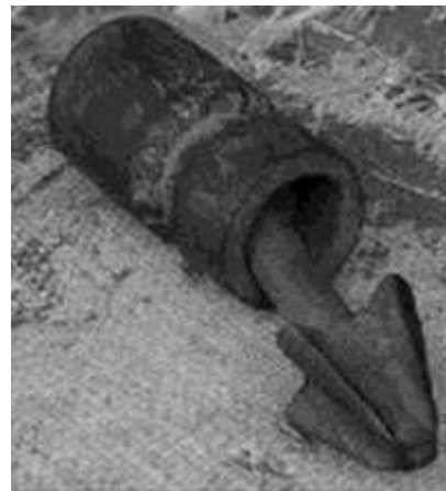
Figure 14. Drill bit with foot valve above
