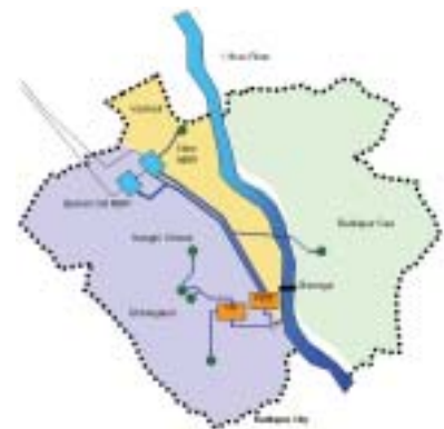
Figure 2.2: Water supply arrangement of Badlapur city.
