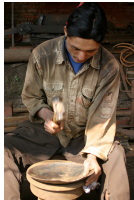
Hammering the blade of a metal runner into the correct shape
