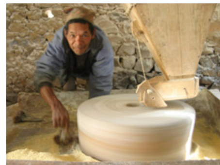
Grinding maize with an improved water mill.
