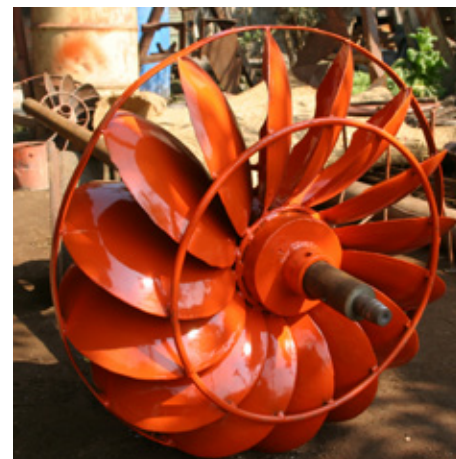
The metal runner for an improved water mill
