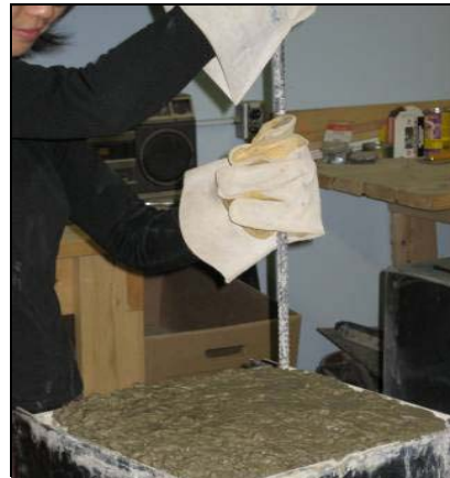
Step 8 - Use a metal rod to help the air escape
