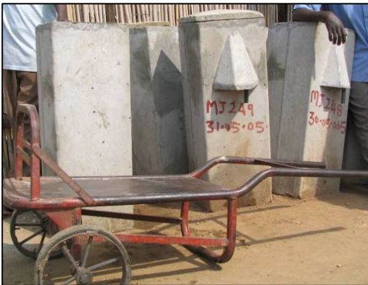
Transporting filters with a specially constructed dolly
