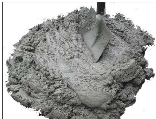
The consistency of the concrete should be fairly stiff and dry. The filter is prone to cracks or leaks if too much water is added.
