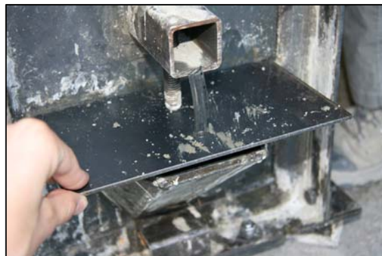
The nose plate should be secured tightly, with the plastic tubing sticking out through the hole
