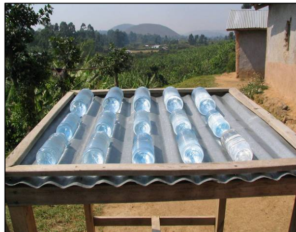
SODIS, or solar disinfection, can be used as part of the multi-barrier approach
