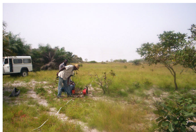
Figure 8: VES Measurement in Nigeria
