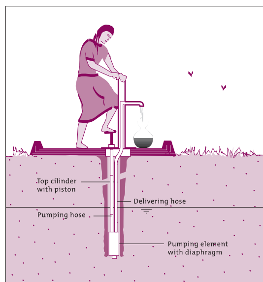
Figure 4.7 Deep-well diaphragm pump
