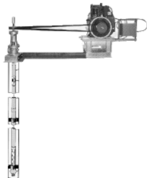
Figure 32 Diesel driven pump
