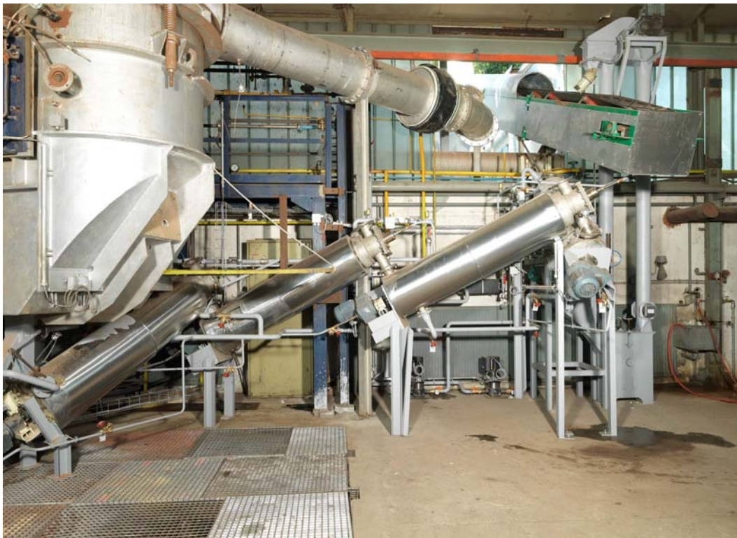
Drum rotary kiln with cooling screw conveyors
