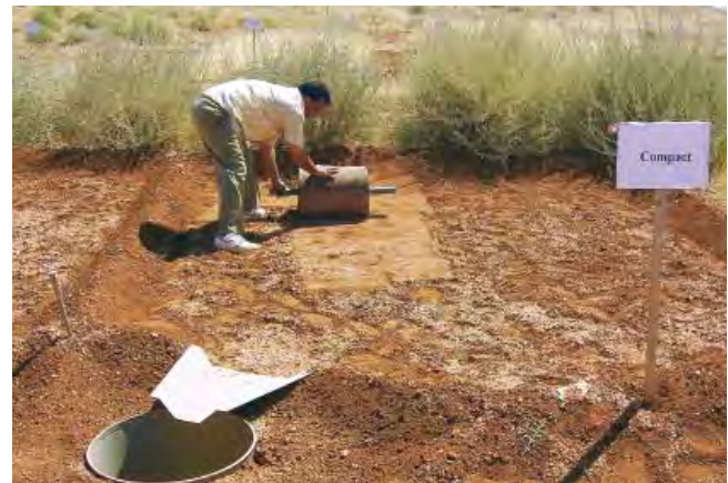
Compaction of micro-catchment surface reduces infiltration, helping to induce runoff.
