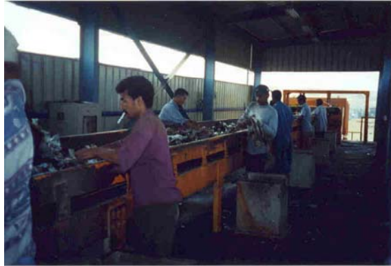
Figure 12.2 Waste recovery sorting line.
