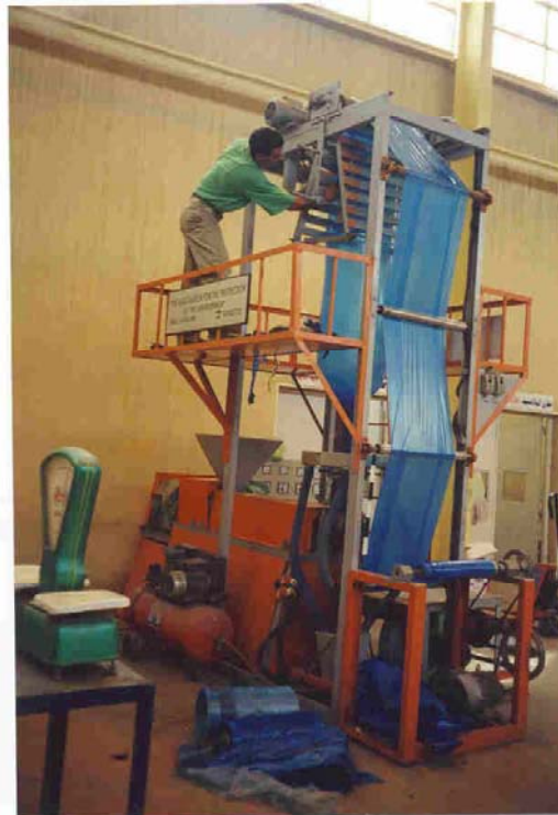
Figure 9.11 Plastic foil manufacturing machine designed and built by the Zabbaleens.
