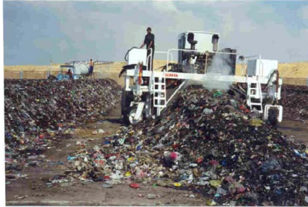
Figure 9.7 The compost turner in action.
