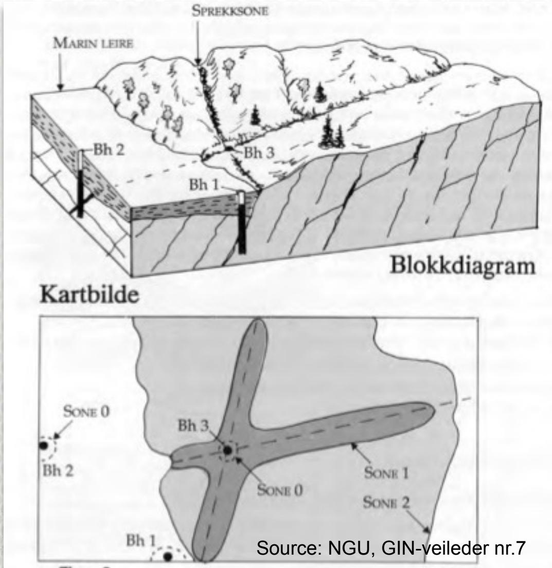
The protection zone for a groundwater supply from a well in bedrock may differ from a well in sediments. In the example to the right the immediate fractures feeding the well constitute Zone 1. Zone 2 is the terrain draining towards the fracture zones.
